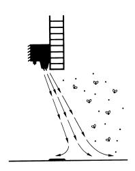
Figure 7 - Desired Air Flow Adjustment for Insect and Dust Control.
